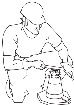
Figure 60-D. Slump Test (Removing Excess Concrete)
